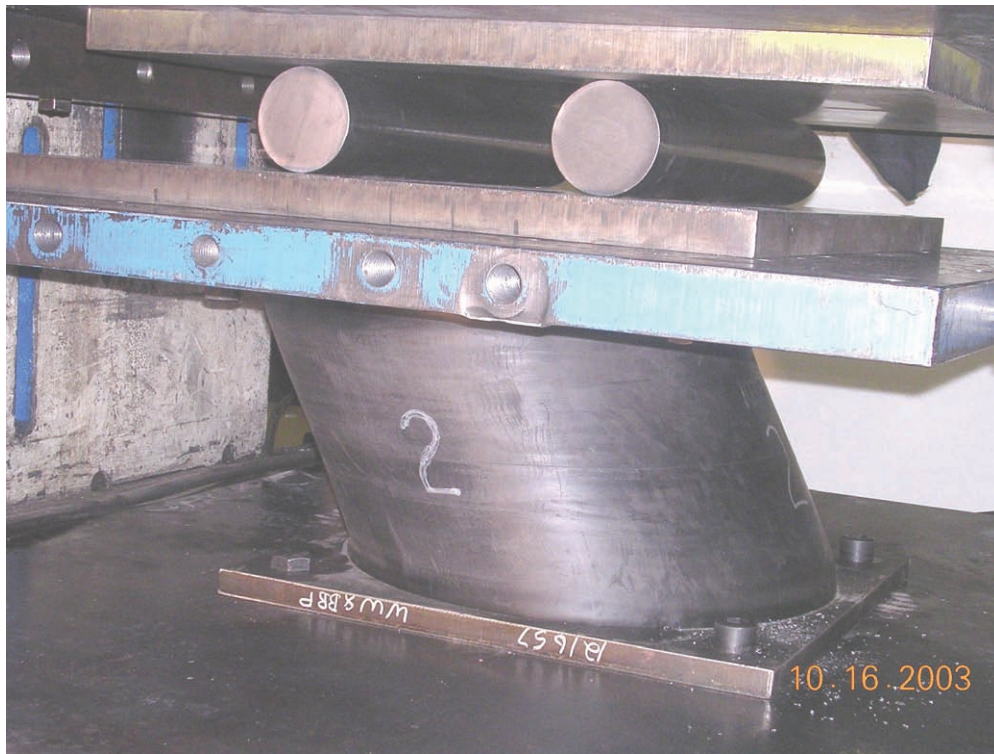
FIGURE 8-14 Lead-Rubber Bearing During High Speed Testing
