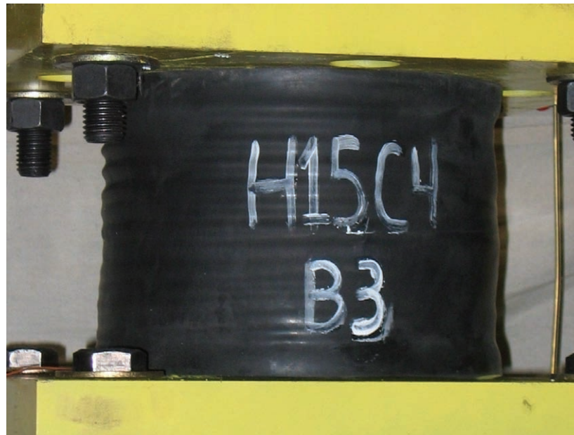
FIGURE 7-14 Rubber Bearing at Tensile Deformation of 60% of the Total Rubber Thickness
