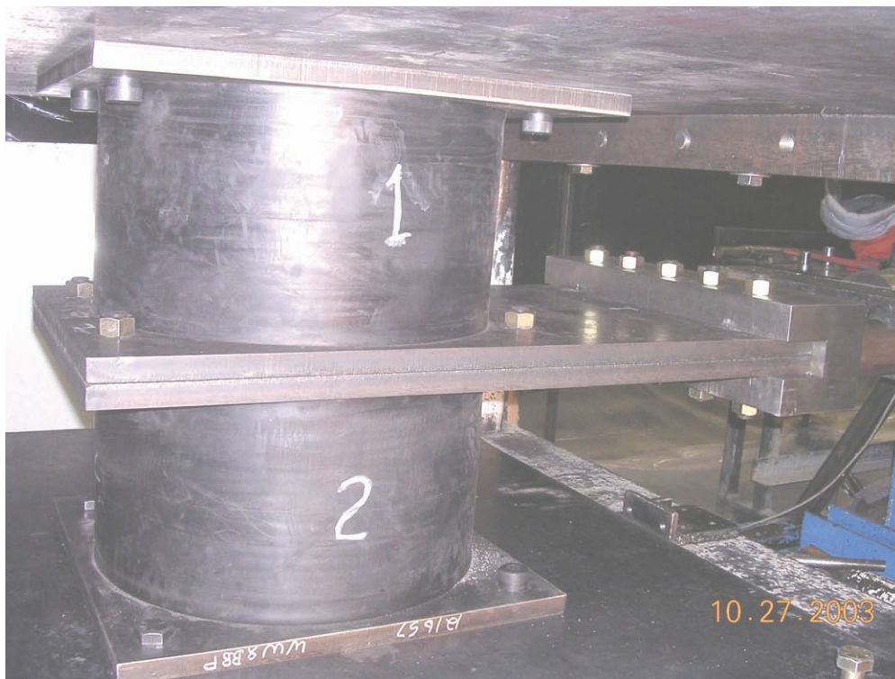
FIGURE 8-15 Lead-Rubber Bearings Tested in Pairs in the 1.6km Cumulative Travel Test
