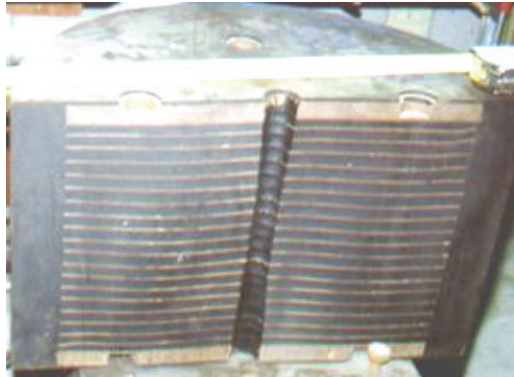
FIGURE 2-10 Section Through an Elastomeric Bearing
