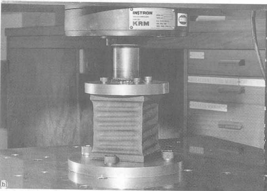
Figure 3.15 (a) Vulcanised laminated-rubber bearing before loading. (b) Vulcanised laminated-rubber bearing under vertical tension. (c) Stress-strain curve for the vulcanised laminated-rubber bearing under both compression and tension. (From Tyler, 1991.)
