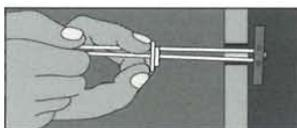
WITH ONE HAND, PULL RING SO METAL CHANNEL RESTS FLUSH BEHIND WALL. SLIDE PLASTIC CAP ALONG STRAPS WITH OTHER HAND UNTIL FLANGE OF CAP IS FLUSH WITH WALL.
