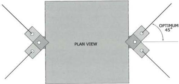
Figure 94: Two-point equipment attachment.
