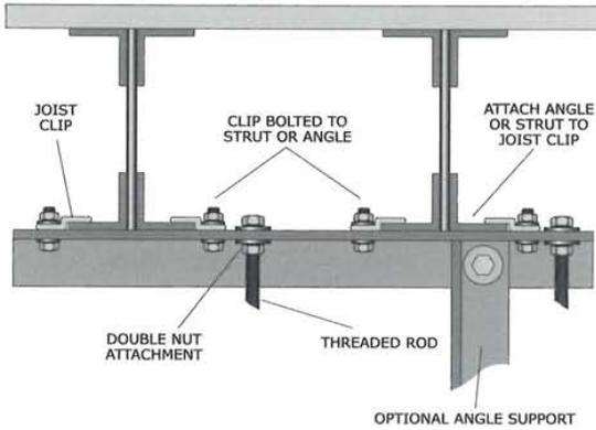
Figure 102: Bar joist construction.
