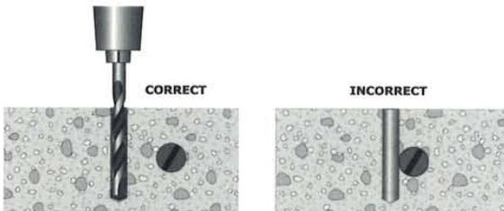
Figure 109: Drilling into concrete with rebar.
