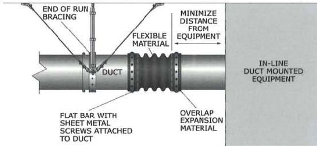
Figure 133: Rubber joint duct connector.
