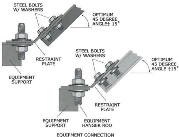
Figure 89: Attachment of angle or strut to the equipment.
