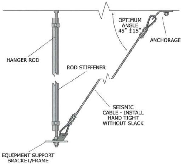
Figure 87: Attachment of cable to the equipment.
