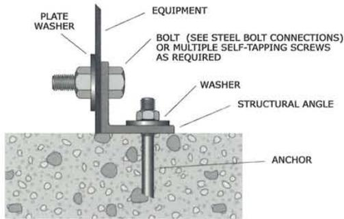
Figure 114: Installing a reinforcing angle bracket to equipment.
