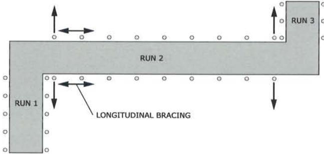
Figure 5: Add longitudinal bracing as necessary.
