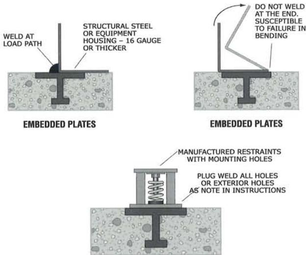
Figure 127: Welding to embedded plates.
