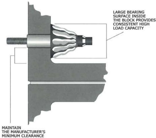
Figure 121: Umbrella anchor in a hollow block wall.
