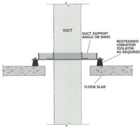
Figure 60: Penetration for interior round duct.
