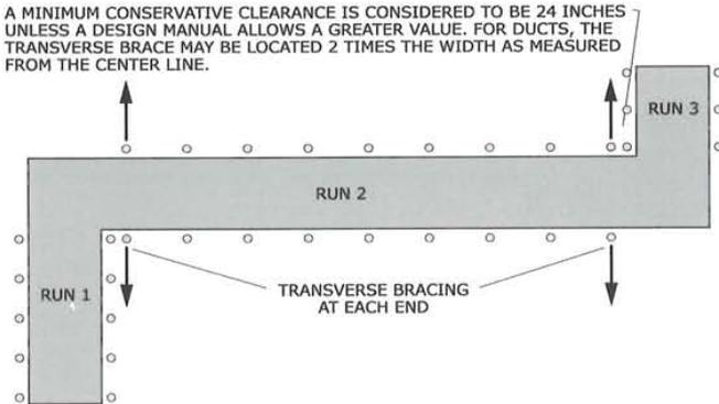
Figure 3: Locate transverse bracing at the ends.
