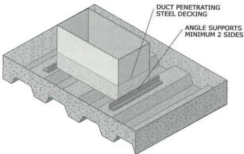
Figure 57: Duct penetration through metal deck roof.
