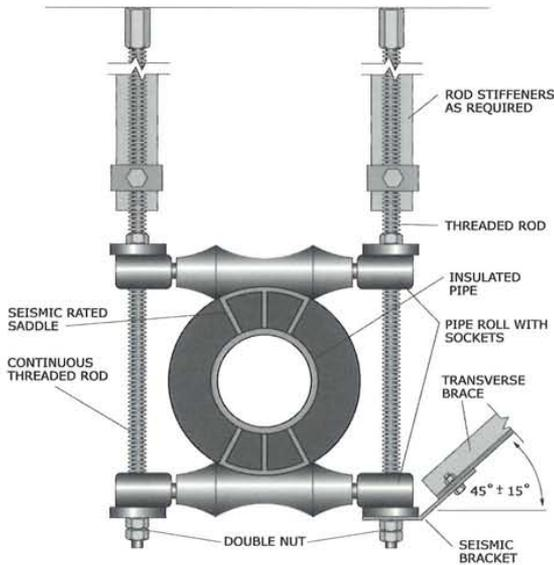
Figure 71: Double roller support for thermally expansive piping.
