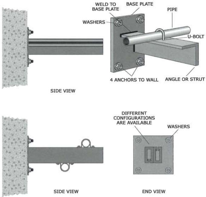
Figure 79: Attachment to the wall with angle or strut welded to attachment plate.
