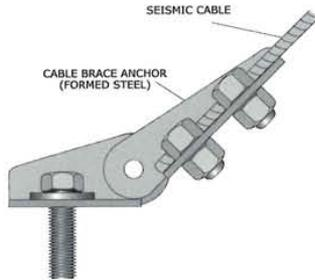
Figure 129: Cable attached with bolts to a bracket.
