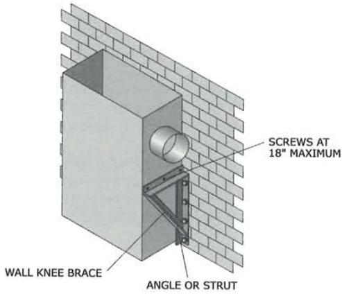
Figure 54: Duct supported by angles.
