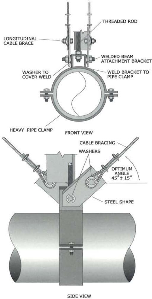
Figure 66: Pipe clamp supports with longitudinal cable brace and hanger rod.
