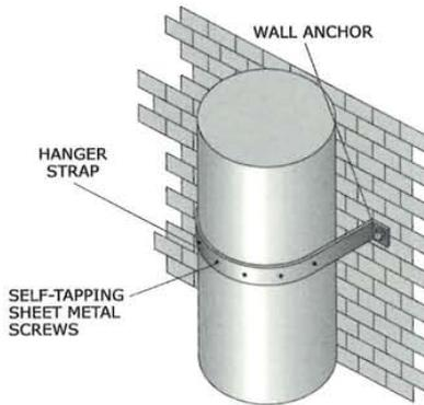
Figure 53: Strap connected directly to wall.
