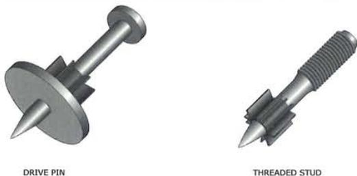
Figure 123: Two types of power-actuated anchors.
