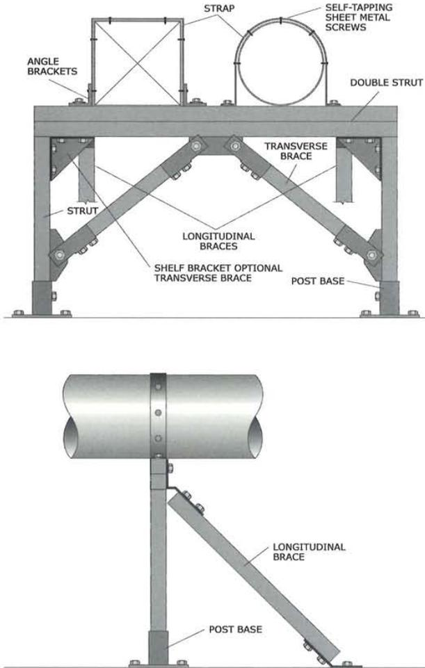
Figure 48: Duct supported off the floor with struts.
