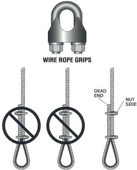
Figure 132: Wire rope grip assemblies.
