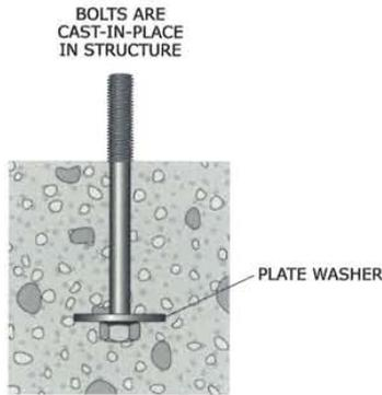
Figure 115: Bolting equipment to cast-in-place anchors.
