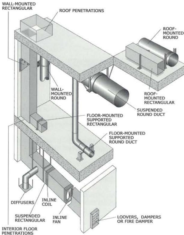
Figure 8: Duct system with different seismic braces.
