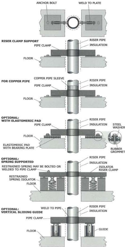
Figure 84: Interior pipe penetration detail.
