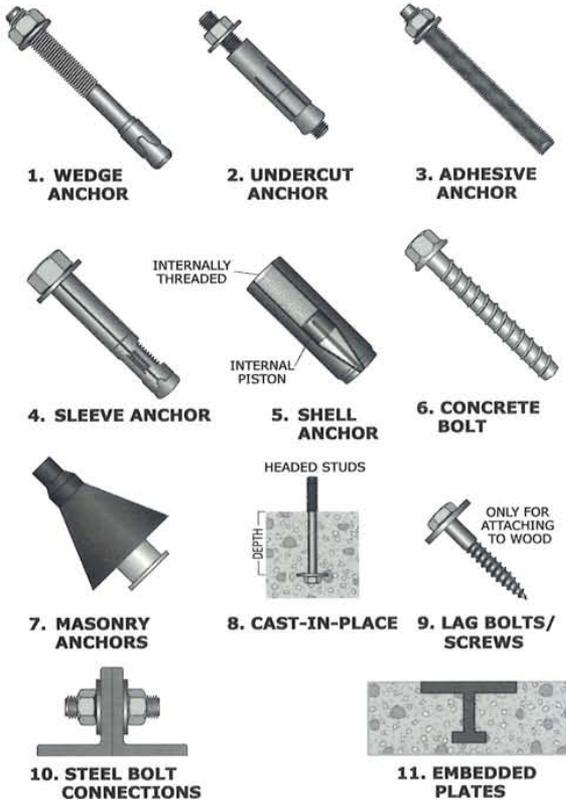
Figure 106: Types of anchors.
