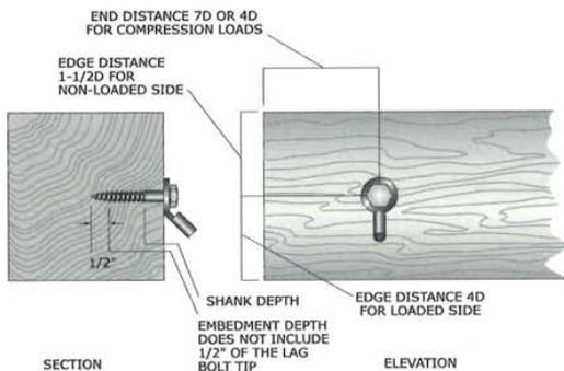
Figure 116: Spacing requirements for wood lag bolts.
