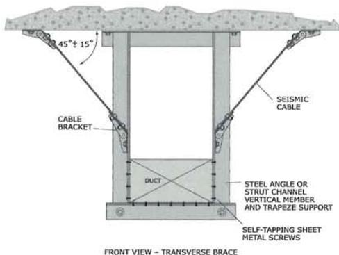
Figure 32: Rectangular duct with steel shapes and braced with cables (transverse).
