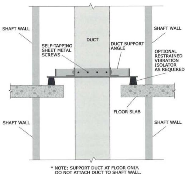
Figure 56: Duct supported in chase.
