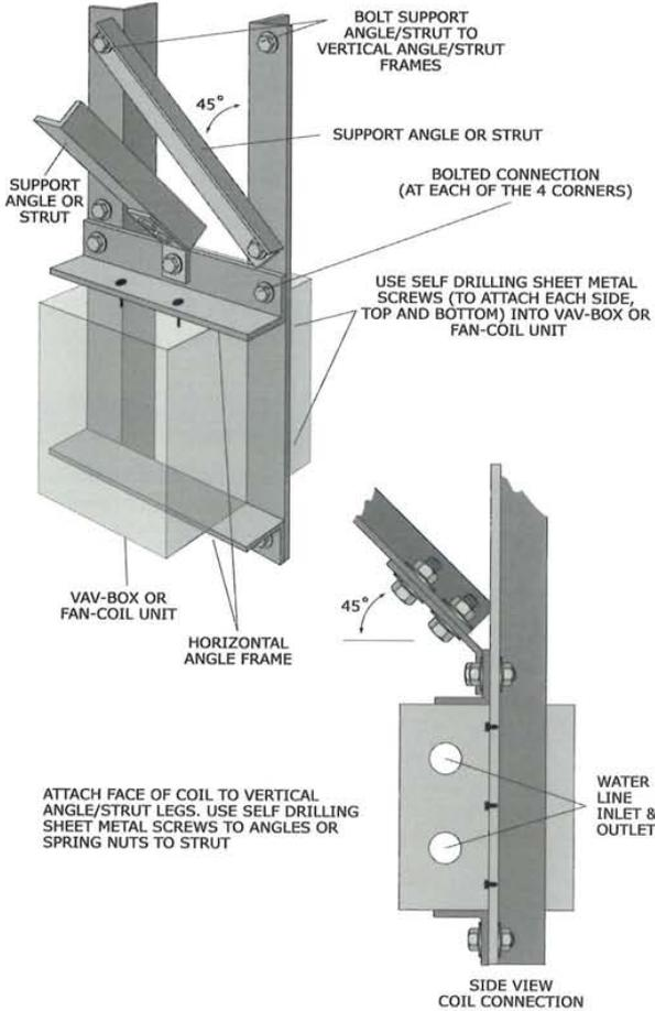
Figure 95: Attachment of double angles for equipment support.
