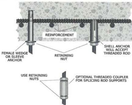
Figure 103: Concrete slab construction.
