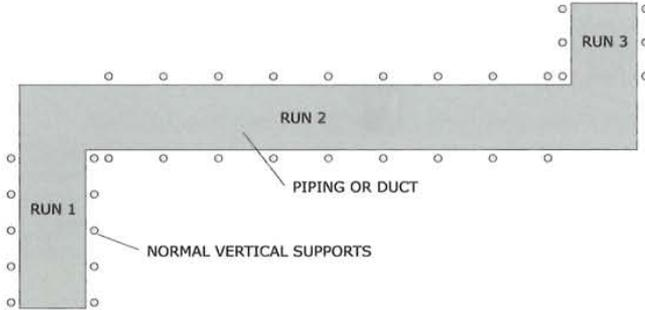
Figure 1: Separate layout into runs.
