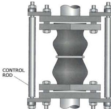
Figure 136: Rubber hose connector with control rods.
