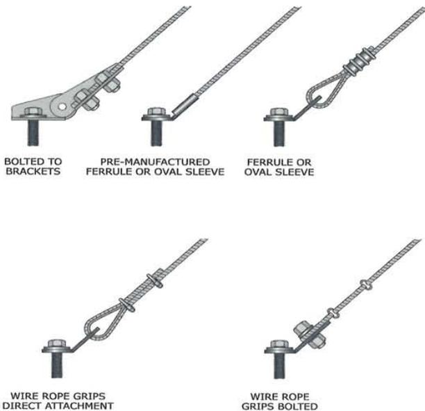
Figure 128: Cable attachments.
