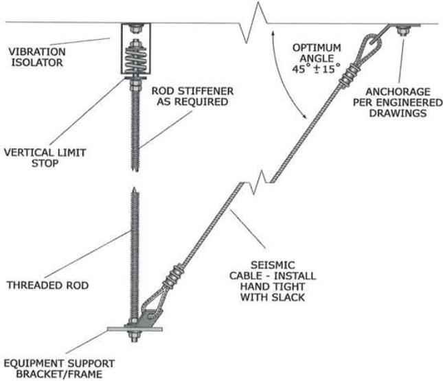
Figure 93: Attachment of cable/rod assembly to the equipment.
