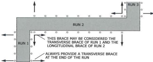
Figure 6: One cost-effective way to rearrange bracing.
