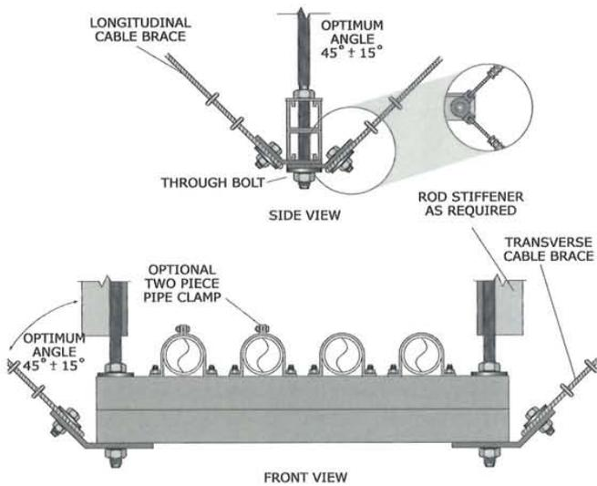
Figure 70: Trapeze support with cable lateral brace.
