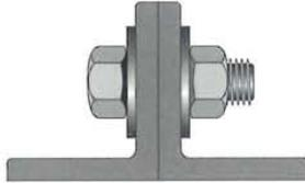
Figure 125: Bolting structural shapes.
