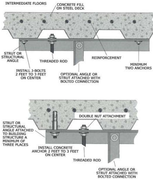
Figure 99: Post-installed anchor; concrete fill on steel deck.
