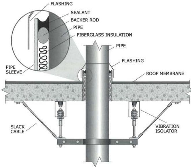
Figure 83: Isolated pipe roof penetration detail.
