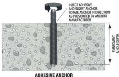
Figure 110: Adhesive anchor installation.
