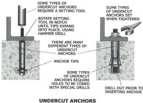
Figure 112: Set undercut anchors.
