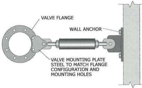
Figure 142: Transverse bracing directly attached to valve.
