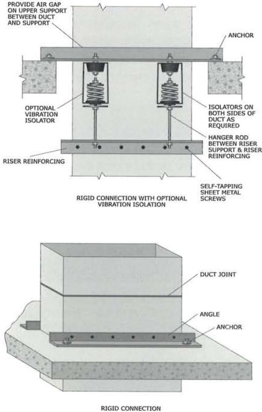
Figure 59: Penetration for interior rectangular duct.
