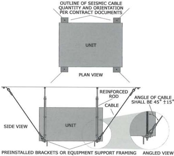
Figure 85: Rigid connection to the building structure.
