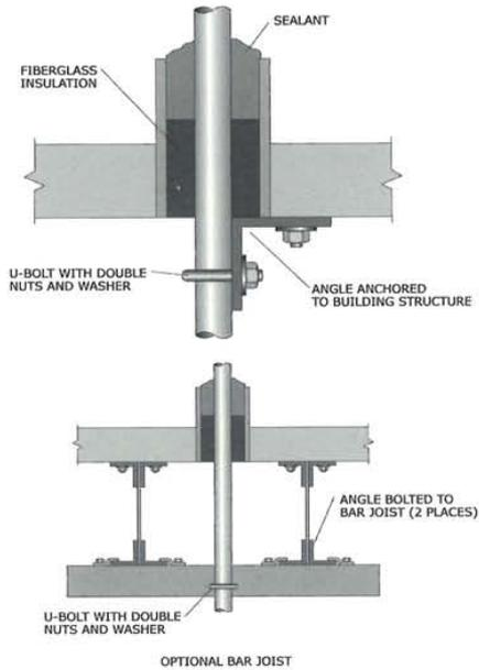
Figure 81: Roof pipe penetration detail.
