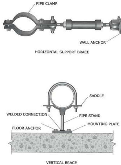
Figure 141: Pipe bracing detail.
