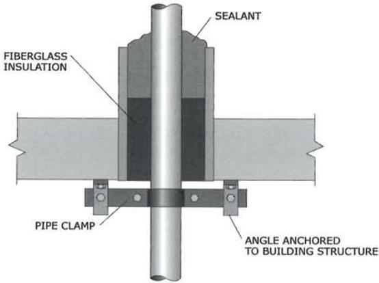
Figure 82: Roof pipe penetration detail.
