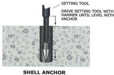
Figure 111: Set shell anchors.
