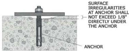
Figure 113: Acceptable gap for grouted plate.
