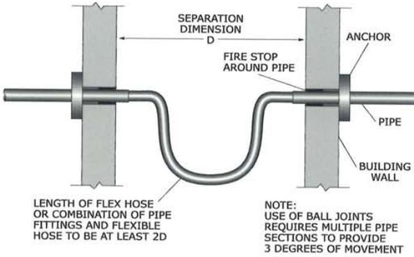
Figure 140: Expansion joint between a separation.
