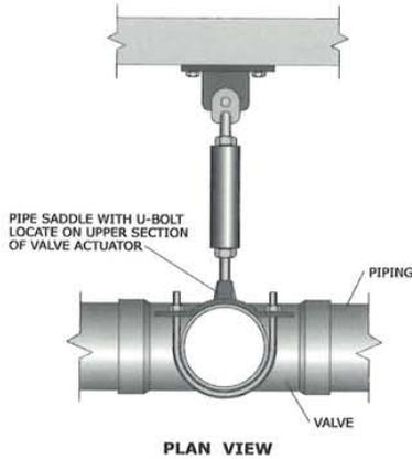
Figure 143: Valve actuator bracing.
