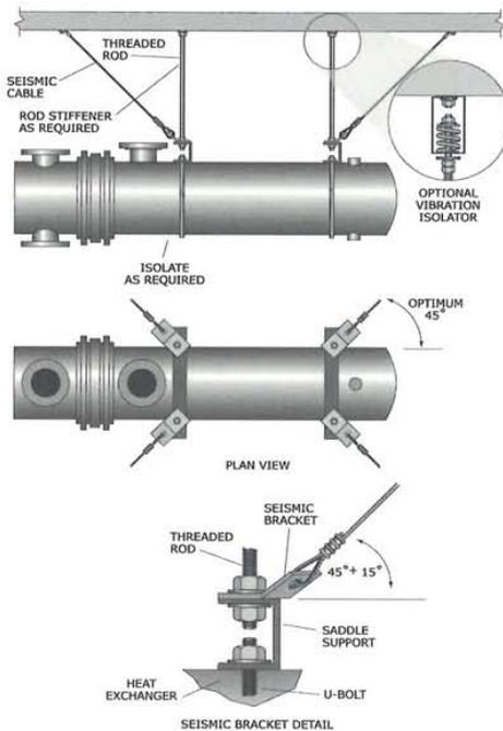
Figure 98: In-line heat exchanger.
