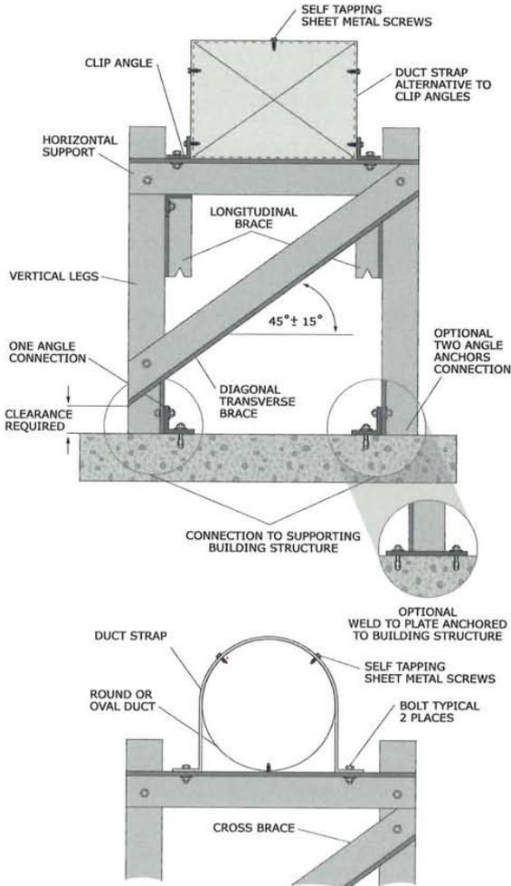
Figure 47: Duct supported off the floor with angles.
