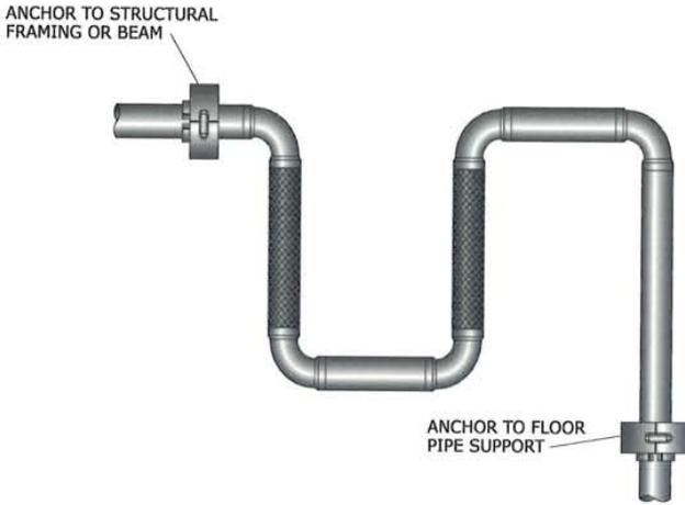
Figure 139: Expansion joint above floor.
