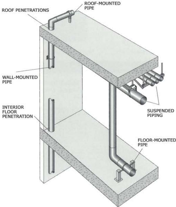
Figure 21: Pipe system with different seismic bracing.
