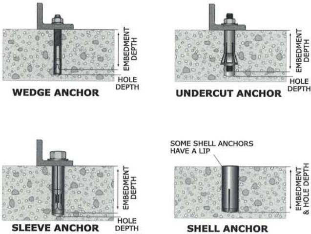
Figure 108: Embedment depth and hole depth of four anchor types.
