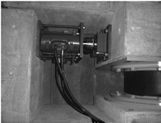
Figure 4.3.21 Static loading test
