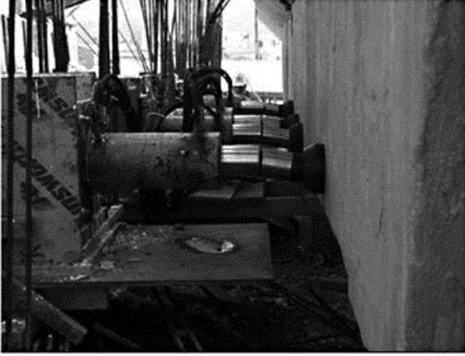
Figure 5.6.13(c) Four hydraulic jacks used in the free vibration test
