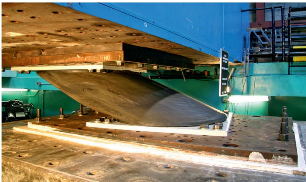
4.3 A bearing for the China Basin Landing office building, San Francisco being tested
