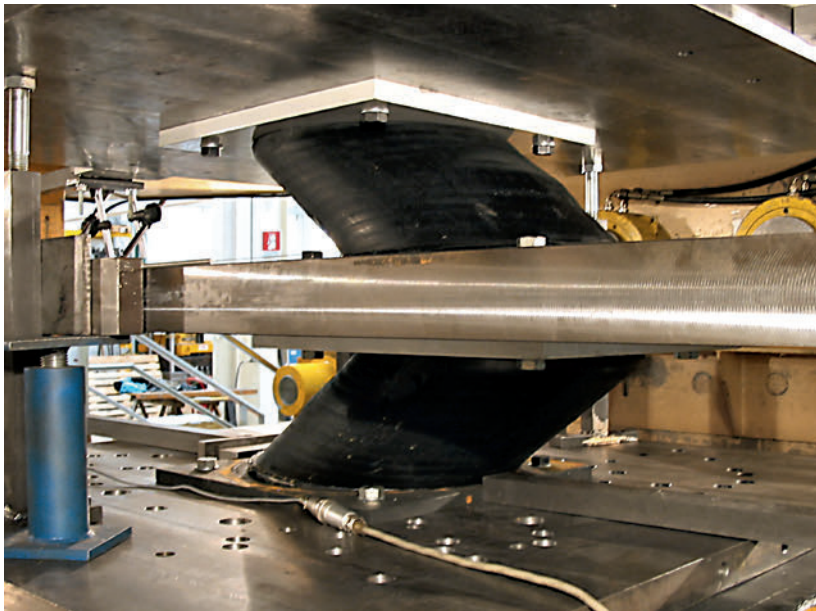
4.2 The testing of elastomeric bearings. Two bearings for the Hospital of Light, Lisbon being tested
