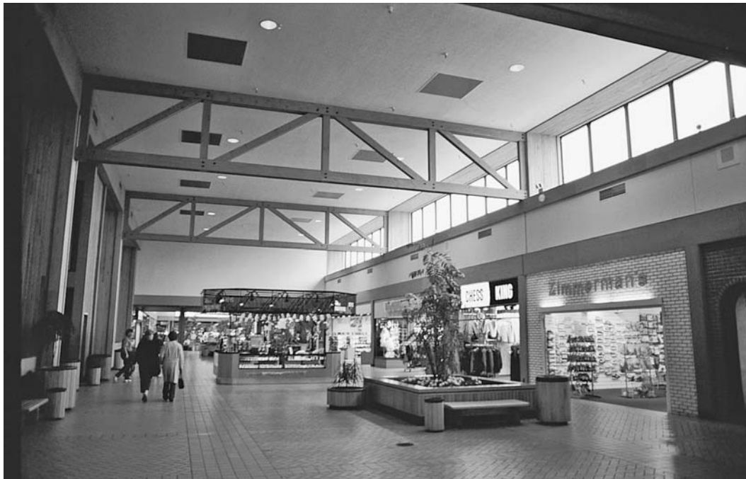
FIGURE 8.13. How far daylight from vertical fenestration penetrates into a room can be clearly seen in this shopping mall. (Photo by Vaughn Bradshaw.)
