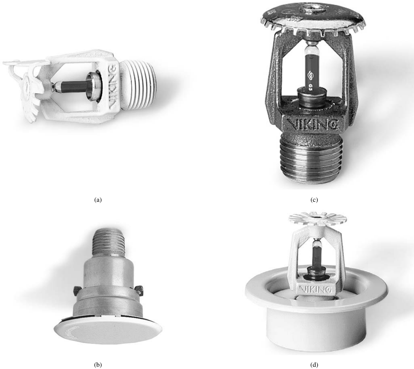
FIGURE 13.13. Sprinkler heads. (a) Sidewall, (b) concealed, (c) upright, and (d) pendant. (Photos courtesy of the Viking Corporation.)
