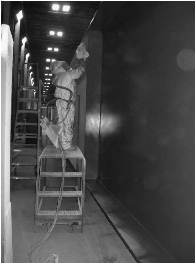
FIGURE 2.9 Roughly half of the steel bridges produced today are painted (the balance are unpainted and comprise weathering steel).
