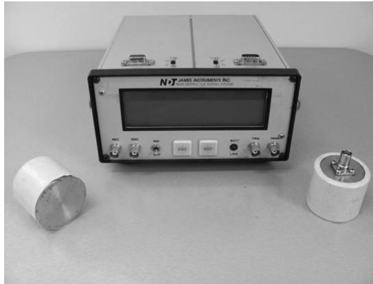
FIGURE 12.12 Photograph of ultrasonic pulse velocity equipment.
