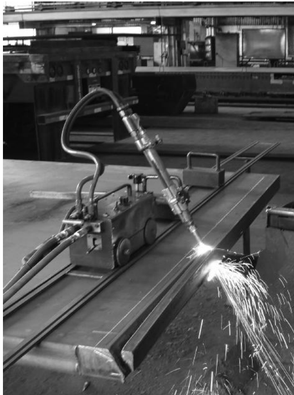
FIGURE 2.5 Oxy-acetylene cutting is shown being used to prepare a plate for welding.
