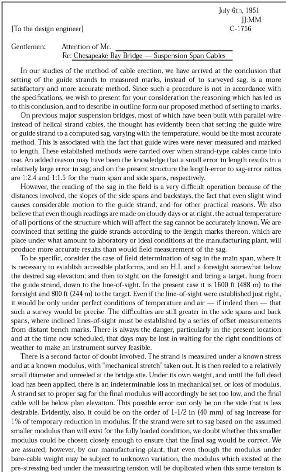
FIGURE 1.7 Setting cable guide strands to marks.
