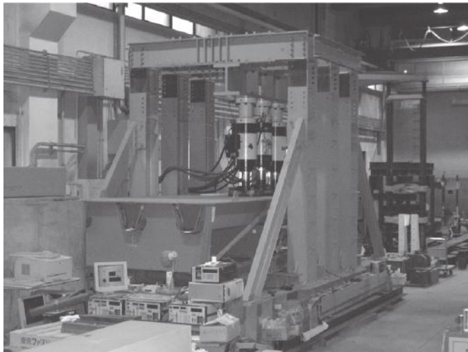
FIGURE 17.73 Three-jack system to simulate moving loads.
