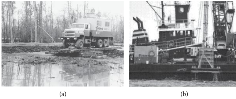
FIGURE 7.5 CPT sounding methods. (a) On land. (b) Over water.
