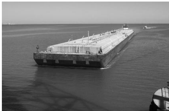
FIGURE 4.6 Tanker barge approaching a bridge. Note the bow depth of at least 1.8 m and the four push knees.
