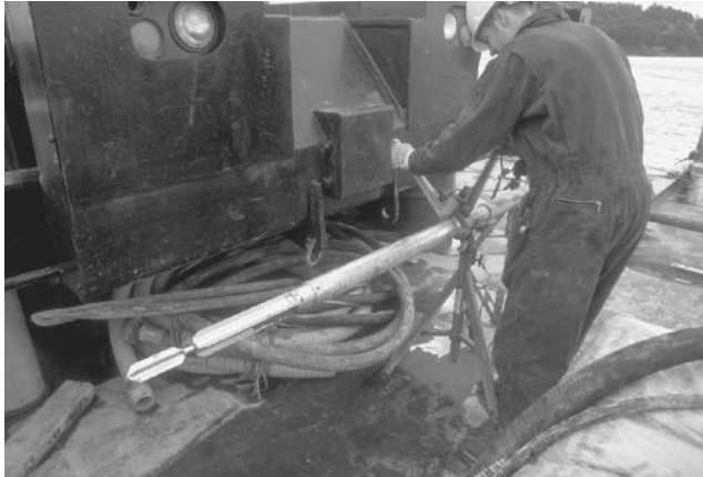
FIGURE 7.7 In situ vane shear device.
